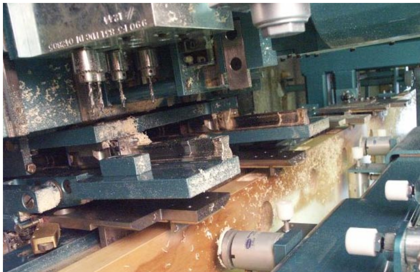
A module called “The Face” is used to drill holes, while a field-installable front seal helps keep sawdust out.
