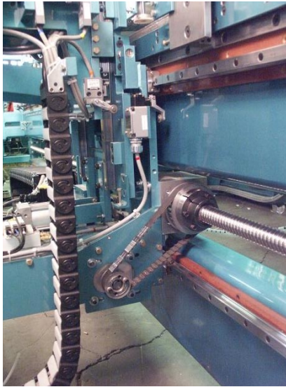
A lubrication system and advanced floating seal improve the rail's service life.
